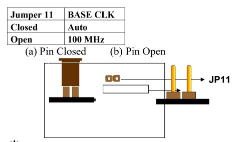
★If you would like to run over 100MHz CPU host bus, like 112 and 124MHz, please set "CPU Clock Frequency" in "CHIPSET FEATURES SETUP" from the BIOS setup screen. If the system can't boot up at CPU frequency that has been set, you can press the 'Insert" key to clear up the set frequency. After restarting the system, it will operate at the default frequency.
