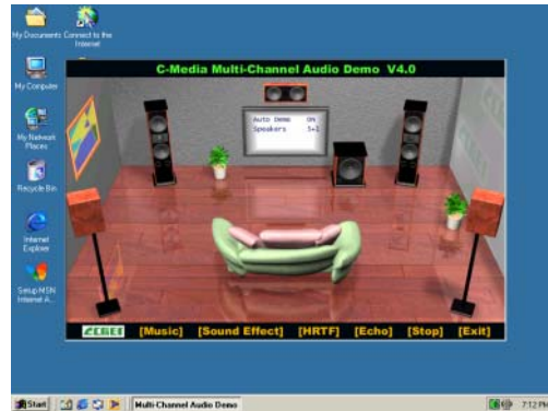
10. Click Start\Program\PCI Audio Application\Multi-Channel Audio Demo to test the 6CH Speaker position
