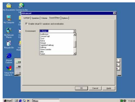
14. By clicking C-Media Mixer\Advanced\Sound Effect selection. You can set up the Sound Environment Simulator
