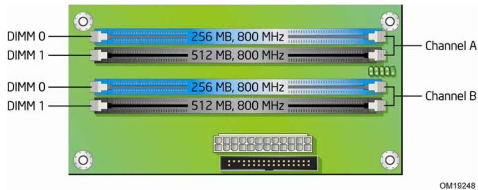
Figure 14. Dual Channel Memory Configuration Example 2
