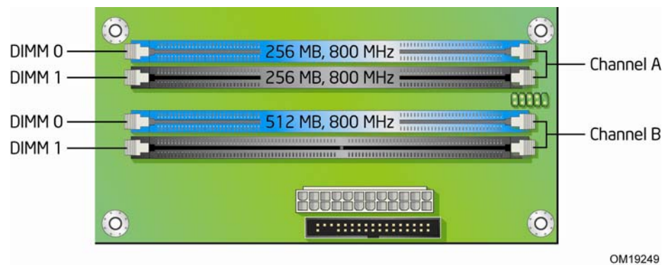
Figure 15. Dual Channel Memory Configuration Example 3
