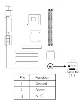
If you are installing a chassis fan in the system unit, connect the fan's connector to location JTI on the system board. The fan will provide adequate airflow throughout the chassis to prevent overheating the CPU.
