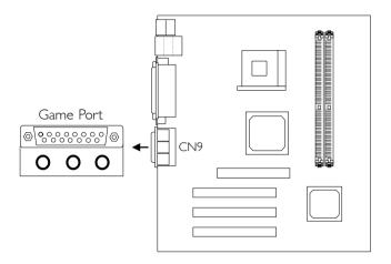
The Game/MIDI port is identical to that of a standard PC game adapter or game I/O port. Connect an analog joystick to the 15-pin D-sub connector (CN9 - Gold) located at the ATX double deck ports of the system board. This port works well with any application that is compatible with the standard PC joystick. You can configure the game port in the Integrated Peripherals submenu ("Super IO Device" field) of the BIOS.
