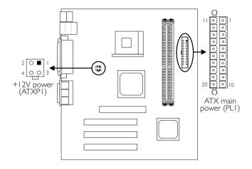
We recommend that you use a power supply that complies with the ATX12V Power Supply Design Guide Version I.I. An ATX12V power supply has a standard 20-pin ATX main power connector and a 4-pin +12V power connector that must be inserted onto PL1 and ATXP1 connectors respectively.
