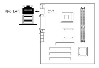
The NB30-BL and NB35-BL system boards are each equipped with an onboard RJ45 fast-ethernet LAN port at location CN7 of the ATX double deck ports. It allows the system board to connect to a local area network by means of a network hub. The Realtek RTL8100 chip that controls this port can be enabled or disabled in the Integrated Peripherals submenu ("Intel OnChip PCI Device" field) of the BIOS. Refer to the Integrated Peripherals section in chapter 3 for more information.
