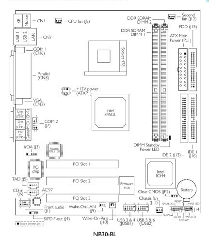
(Uses the Intel® 845GL chipset and supports onboard LAN)
