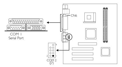
The built-in serial ports are RS-232C asynchronous communication ports with I6C550A-compatible UARTs that can be used with modems, serial printers, remote display terminals, and other serial devices. You can select the serial ports' I/O address in the Integrated Peripherals submenu ("Onboard Super IO Device" field) of the BIOS.
