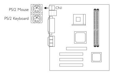
The system board is equipped with an onboard PS/2 mouse (Green) and PS/2 keyboard (Purple) ports - both at location CNI of the ATX double deck ports of the system board. The PS/2 mouse port uses IRQ12. If a mouse is not connected to this port, the system will reserve IRQ12 for other expansion cards.
