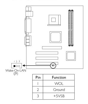
The Wake-On-LAN function is applicable only when you are using a LAN add-in card that has the same function. It will allow the network to remotely power-on a Soft Power Down (Soft-Off) PC. However, if your system is in the Suspend mode, you can power-on the system only through an IRQ or DMA interrupt.
