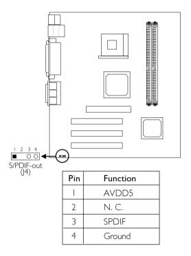
The system board is equipped with the S/PDIF (Sony/Philips Digital Interface) digital audio interface. S/PDIF is a standard audio file transfer format that transfers digital audio signals to a device without having to be converted first to an analog format. This prevents the quality of the audio signal from degrading whenever it is converted to analog.
