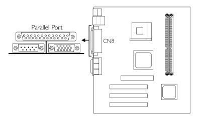
The system board has a standard parallel port (CN8 - Burgundy) located at the ATX double deck ports of the board for interfacing your PC to a parallel printer. It supports SPP, ECP, EPP and PntMode modes. You can select the port's mode in the Integrated Peripherals submenu ("Onboard Super IO Device" field) of the BIOS.
