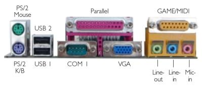
ATX Double Deck Ports on NB30-BC and NB35-BC
