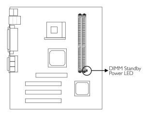
The DIMM Standby Power LED will turn red when the system's power is on or when it is in the Suspend state (Power On Suspend or Suspend to RAM). It will not light when the system is in the Soft-Off state.
