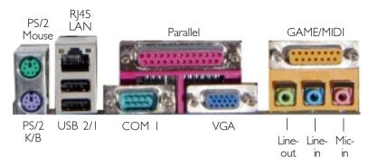
ATX Double Deck Ports on NB30-BL and NB35-BL
