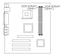
The system board is equipped with two 184-pin DDR SDRAM DIMM (Dual In-line Memory Module) sockets that support 2.5V DDR SDRAM DIMM. Double Data Rate SDRAM (DDR SDRAM) is a type of SDRAM that doubles the data rate through reading and writing at both the rising and falling edge of each clock. This effectively doubles the speed of operation therefore doubling the speed of data transfer.
