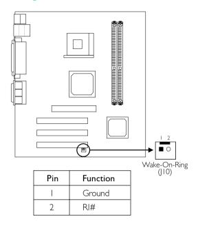
The Wake-On-Ring connector is used to connect to an internal modem add-in card that has the same connector. It will allow the system that is in the Suspend mode or Soft Power Off mode to wake-up/power-on to respond to calls coming through the internal modem card.
