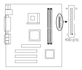
The system board is equipped with a shrouded floppy disk drive connector that supports two standard floppy disk drives. To prevent improper floppy cable installation, the shrouded floppy disk header has a keying mechanism. The 34-pin connector on the floppy cable can be placed into the header only if pin I of the connector is aligned with pin I of the header. You can enable or disable this function in the Integrated Peripherals submenu ("Onboard Super IO Device" field) of the BIOS.
