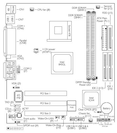
NB30-BC (Uses the Intel® 845GL chipset)
