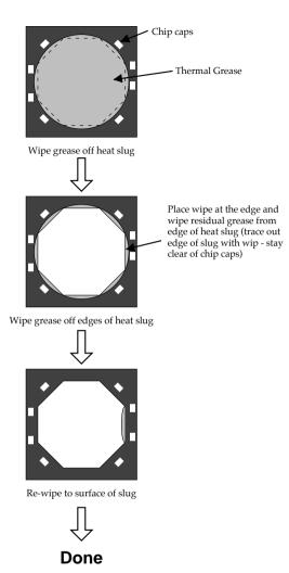
Figure 2–8. Grease Removal Process
