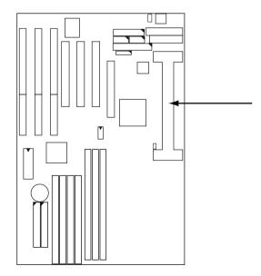
The retention clip should be inserted so that the small rectangle window is more toward to the right hand side of the board.
