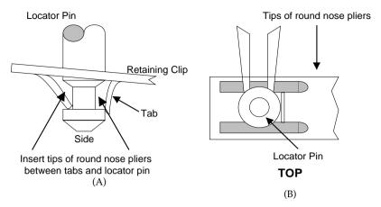
Figure 2–7. Round-nose pliers insertion points (a) side view (b) top view
