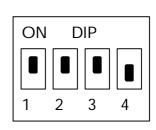
DIP switch, ( ex. : ON,ON,ON,OFF) O N : switch to the 'ON' position. OFF : switch to the 'OFF' position.
