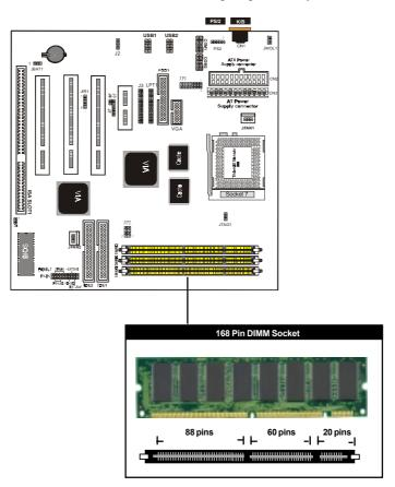
The Dual Inline Memory Module (DIMM) memory module must be 3.3v Extended Data Output (EDO) DRAM or SDRAM. You can identify the type of DIMM module by the illustration below:
