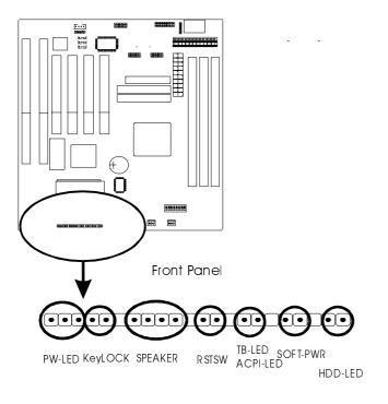
*PW-LED* is a 3-pin connector. It is used to connect to the LED on the case front panel. The LED shows the status of the power.
