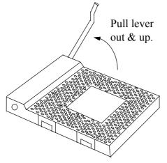
2.Align the CPU and socket pin 1 corners. Match the processor corner containing the blunt edge and the white dot to the socket corner with the distinctive pin arrangement. The pins on the bottom should align with the inner 3 rings of holes in the socket, then place the CPU in the socket. It should insert easily. If it doesn't, pull the level up a little more.
