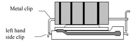
3. Hook the left hand side clip on the CPU socket first.
