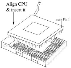
3.Press the lever down. The plate will slide forward. You will feel some resistance as the pressure starts to secure the CPU in the socket. When the CPU is installed, the lever should snap into place at the side of the socket.
