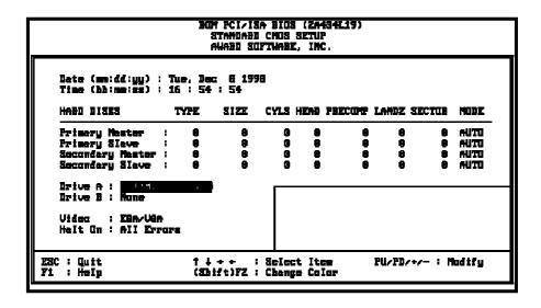
The "Standard CMOS Setup" allows user to configure system setting such as current date and time, type of hard disk drive installed in the system, floppy drive type, and the type of display monitor. Memory size is auto detected by the BIOS and displayed for your reference. When a field is highlighted (direction keys to move cursor and <Enter> key to select). The entries in the field will be changed by pressing <PageDown> or <PageUp> key or user can enter new data directly from the keyboard.
