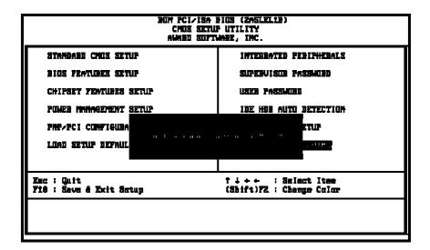
The "Quit Without Saving" option will bring you back to normal boot up procedure without saving any data into CMOS RAM. All of the old data in the CMOS will not be destroyed.
