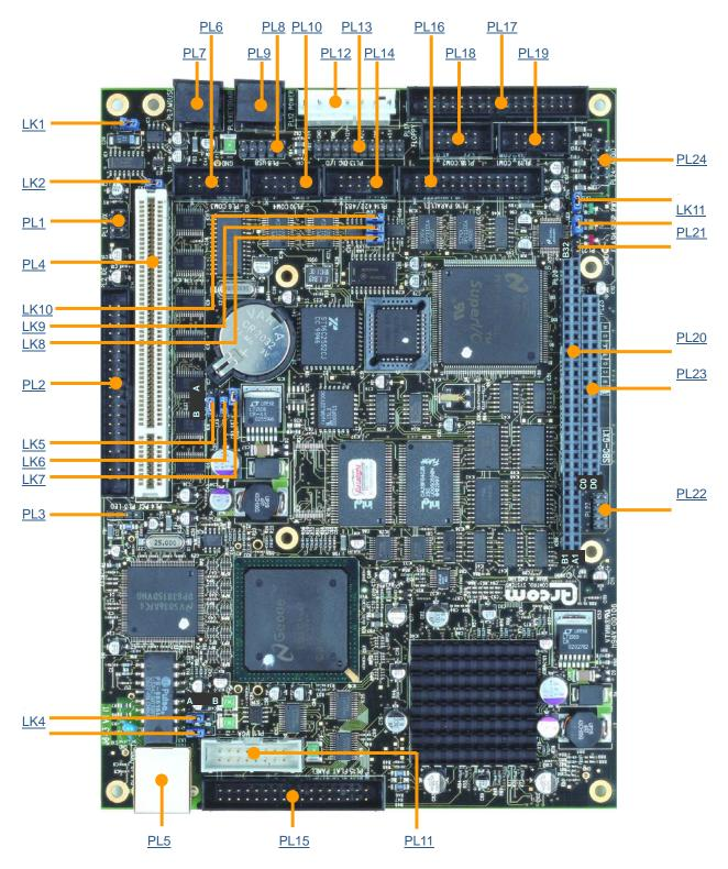
The following diagram shows the connectors on the back of the SBC-GX1:
