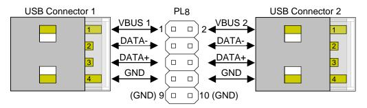
A USB power control switch is used to control the power and protect against short circuit conditions. This can be enabled/disabled by the processor and the USB function needs to be enabled in the BIOS to ensure that power is supplied to each device. The USB feature is controlled using the <u>Chipset features setup</u> screen within the Setup utility - see page <u>34</u> for details.
