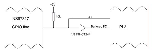
The NS97317 GPIO lines must be configured using the registers built into the device to ensure they function correctly. Various features can be programmed for each pin, including direction control and pull up/down resistors. As the GPIO lines also share pins with dedicated functions these must be disabled if the line is to be used.
