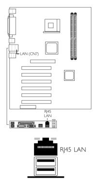
The NB60-EL and NB76-EA system boards are each equipped with an onboard RJ45 fast-ethernet LAN port at location CN7 of the ATX double deck ports. It allows the system board to connect to a local area network by means of a network hub. The Realtek RTL8100 chip that controls this port can be enabled or disabled in the Integrated Peripherals submenu ("Intel OnChip PCI Device" field) of the BIOS. Refer to the Integrated Peripherals section in chapter 3 for more information.
