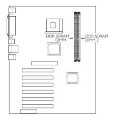
The system board is equipped with two 184-pin DDR SDRAM DIMM (Dual In-line Memory Module) sockets that support 2.5V DDR SDRAM DIMM. Double Data Rate SDRAM (DDR SDRAM) is a type of SDRAM that doubles the data rate through reading and writing at both the rising and falling edge of each clock. This effectively doubles the speed of operation therefore doubling the speed of data transfer.
