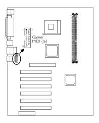
The system board is equipped with a 15-pin connector at location J6 for connecting an external game/MIDI port. One card-edge bracket, mounted with a serial port cable and a game/MIDI port cable, is provided with the system board. Install the card-edge bracket to the system chassis then connect the game/MIDI port cable to connector J6. Make sure the colored stripe on the ribbon cable is aligned with pin I of connector J6.
