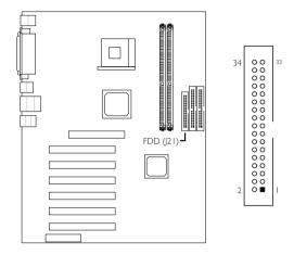
The system board is equipped with a shrouded floppy disk drive connector that supports two standard floppy disk drives. To prevent improper floppy cable installation, the shrouded floppy disk header has a keying mechanism. The 34-pin connector on the floppy cable can be placed into the header only if pin I of the connector is aligned with pin I of the header. You may enable or disable this function in the Integrated Peripherals submenu ("Onboard Super IO Device" field) of the BIOS.
