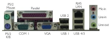
ATX Double Deck Ports on NB76-EA and NB60-EL
