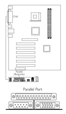
The system board has a standard parallel port (CN6 - Burgundy) located at the ATX double deck ports of the board for interfacing your PC to a parallel printer. It supports SPP, ECP, EPP and PntMode modes. You can select the port's mode in the Integrated Peripherals submenu ("Onboard Super IO Device" field) of the BIOS.
