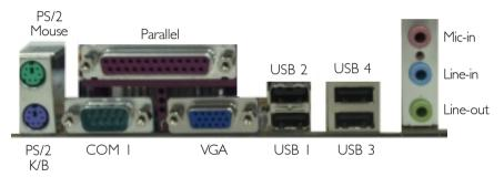
ATX Double Deck Ports on NB76-EC and NB60-EC
