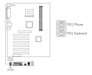
The system board is equipped with an onboard PS/2 mouse (Green) and PS/2 keyboard (Purple) ports - both at location CN4 of the ATX double deck ports of the system board. The PS/2 mouse port uses IRQ12. If a mouse is not connected to this port, the system will reserve IRQ12 for other expansion cards.
