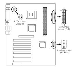
We recommend that you use a power supply that complies with the ATX12V Power Supply Design Guide Version 1.1. An ATX12V power supply has a standard 20-pin ATX main power connector, a 4-pin +12V power connector and a 6-pin auxiliary power connector that must be inserted onto PLI, ATXP1 and ATXP2 connectors respectively.
