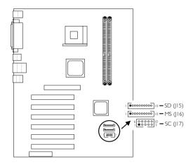
The system board is equipped with a security interface - Smart Card (SC) interface and two compact storage interfaces - Memory Stick (MS) interface and Secure Digital Memory Card (SD) interface. Use the optional Smart I/O drive to insert these cards.
