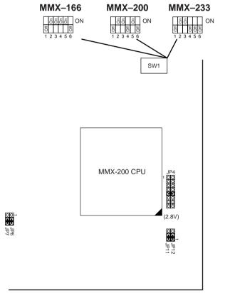
Figure 2–1. CPU Type Configuration
