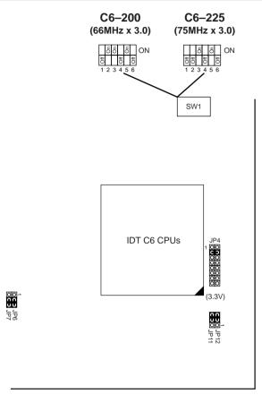
Figure 2–5. CPU Type Configuration
