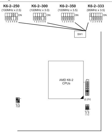
Figure 2–3. CPU Type Configuration
