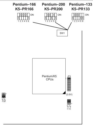
Figure 2–6. CPU Type Configuration
