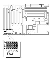
Voltage Auto-setting -- Inserting jumper pack on jumper group row B/C of SW2. Setting to AUTO on " CPU Voltage" item in Chipset
