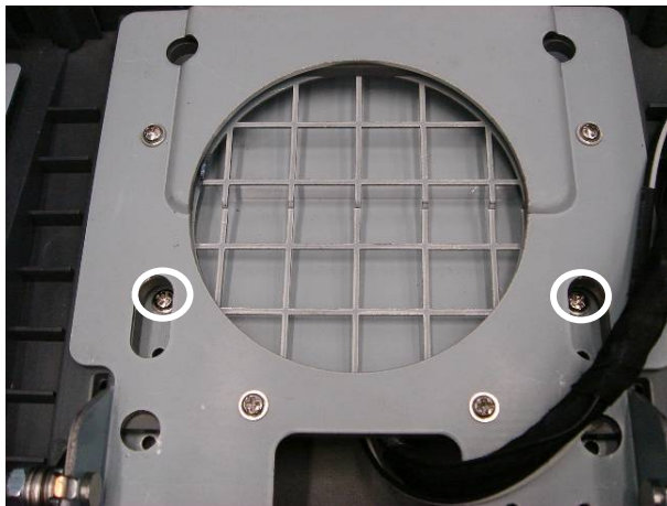
e. Remove the screws (2).
