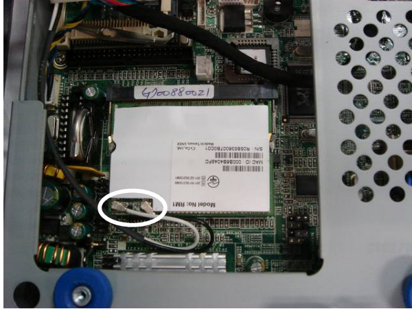
a. Disconnect the antenna (2).
