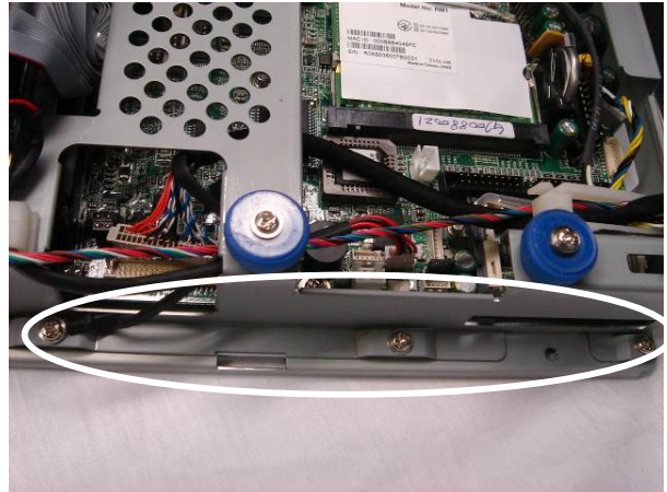
f. Remove the screws (3) to remove the EMI shielding box.
