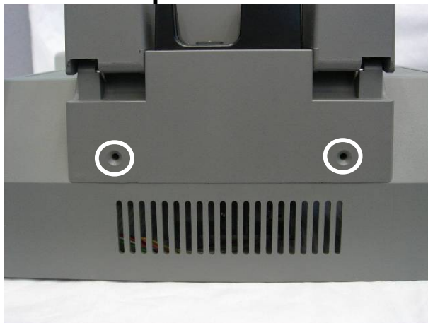
a. Remove the screws (2).
