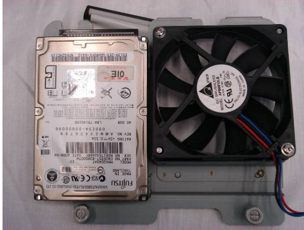
a. Remove the HDD drive bracket.
