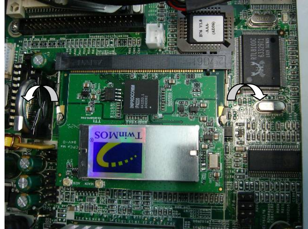
b. To remove the Mini PCI card, release the two metal latches as shown in the picture until the card pops up. Remove the Mini PCI card from the slot.
