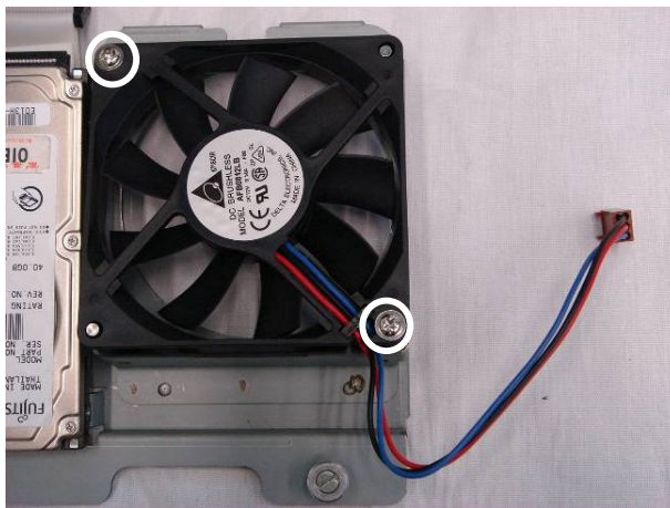
c. Remove the screws (2) to replace the fan.
