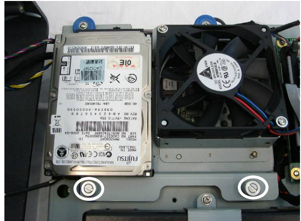
d. Loosen the screws (2) to lift the HDD drive bracket up.
