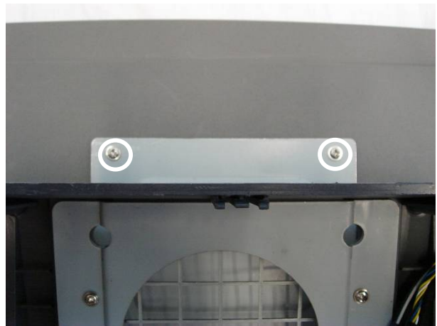
f. Remove the screws (2).
