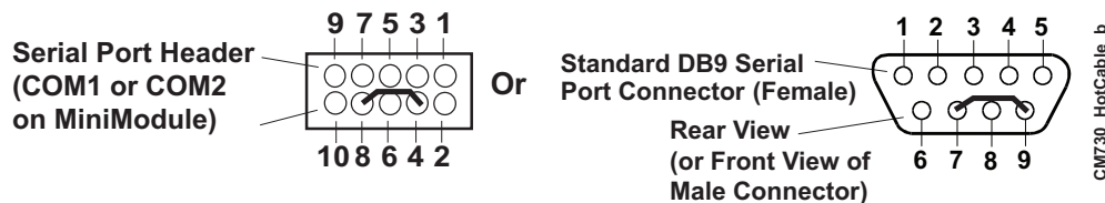
Figure 3-2. Hot Cable Jumper
