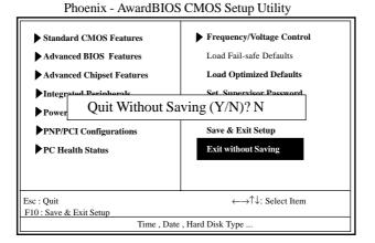
Typing "Y" will quit the Setup Utility without saving to RTC CMOS RAM.
