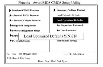
Pressing 'Y' loads the default values that are factory settings for optimal performance of system operations.
