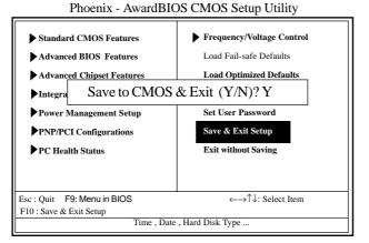
Typing "Y" will quit the Setup Utility and save the user setup value to RTC CMOS RAM.
