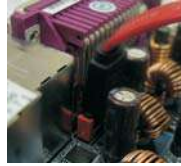
Connect the SATA data cable to the eSATAII connector (eSATAII)
