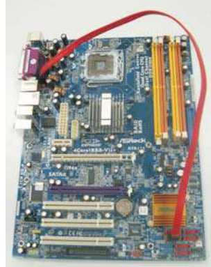
Connect the SATA data cable to the eSATAII connector (eSATAII)
