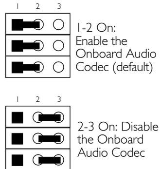
If you are not using the onboard audio codec, set pins 2 and 3 to On (Disabled) and set the “OnChip Sound” field in the Advanced Chipset Features submenu of the BIOS to Disabled.
