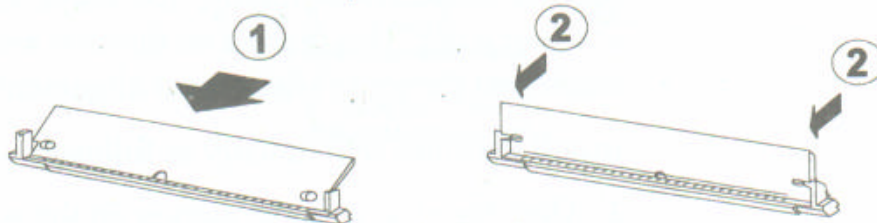
Figure 3-2. Installing a SIMM Module
