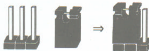
Figure 2 - 1. Jumper with Pins Shorted
