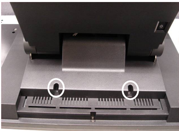
c. Remove the screws (2).
