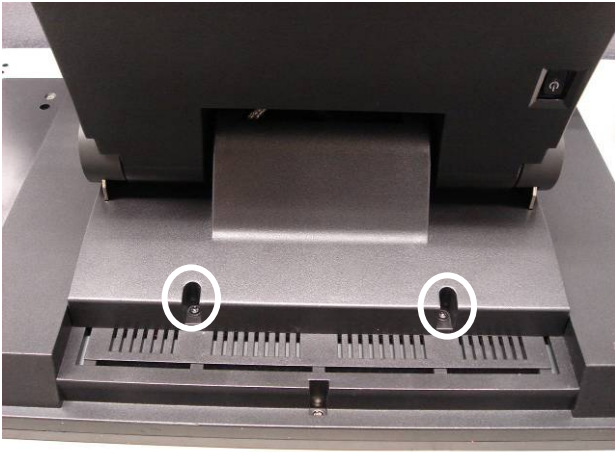
c. Remove the screws (2).
