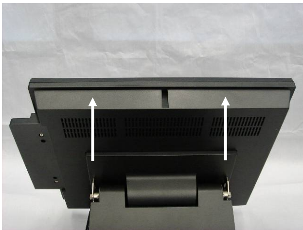
e. Lift the LCD module up.
