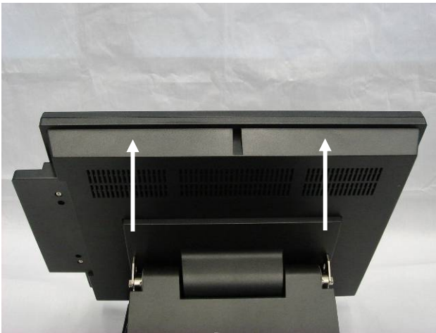
e. Lift the LCD module up.
