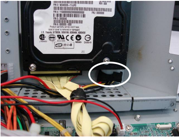
c. Disconnect the cable (1) to replace the HDD.
