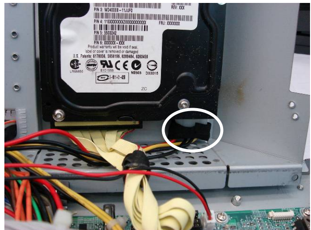
d. Disconnect the cable (1).
