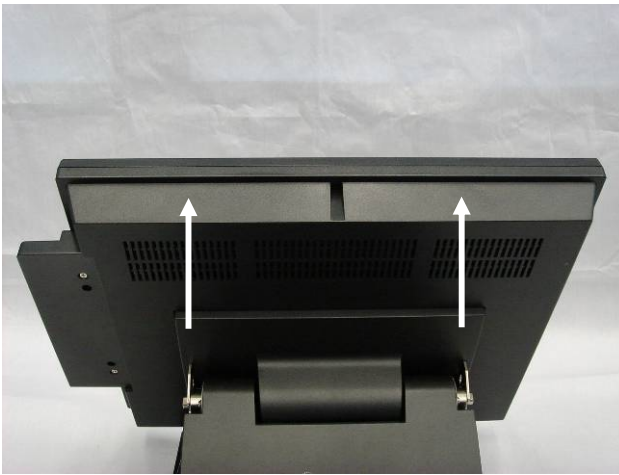
e. Lift the LCD module up.
