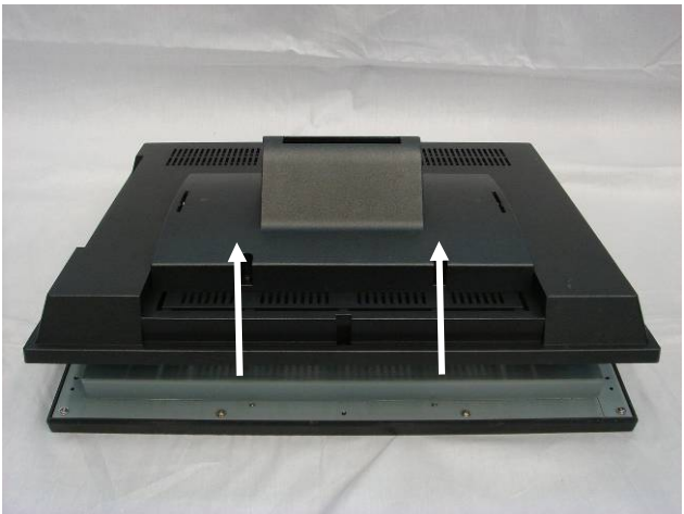
l. Lift the LCD cover up.
