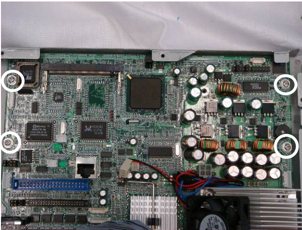
e. Remove the screws (4).
