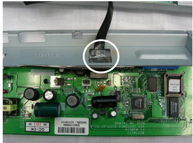
r. Pass the cable through the front bracket and then connect the cable (1) to the MSR board.
