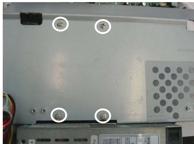
b. Remove the screws (4).
