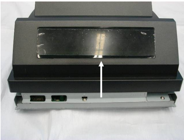
g. Lift the base cover up and remove it.
