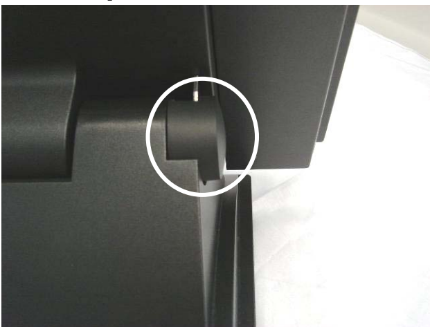
a. Remove the hinge covers on both sides using a screwdriver or finger to push the clip.
