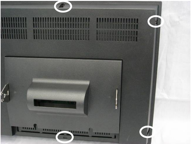
j. Remove the screws (4).
