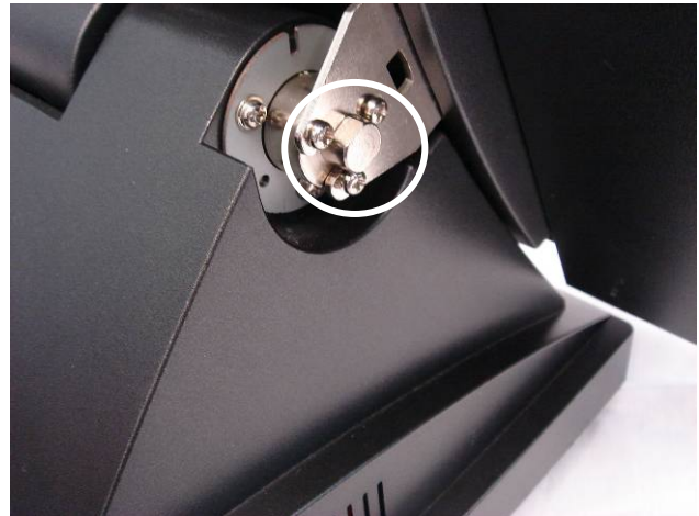
b. Remove the screws (6) (three on each side).
