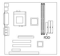
2. Install the other 34-pin header connector(s) into
