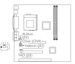
devices such as voice modem cards. By installing a PCI voice modem card that is also equipped with a TAD connector, connect one end of the cable (that came with the card) to the card's TAD connector and the other end to the TAD connector on the system board. The voice modem will interface with the onboard audio allowing voice to come from the external speaker.
