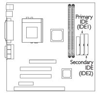
2. Install the other 40-pin header connector(s) into the device with the colored edge of the ribbon cable aligned with pin 1 of the drive edge connector(s).
