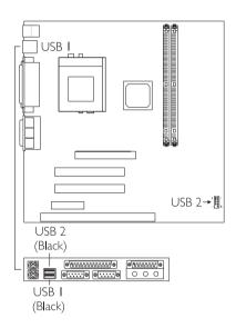
system board allows you to connect the optional 3rd and 4th USB ports. These optional USB ports, which are mounted on a card-edge bracket, will be provided as an option. If you wish to use the optional 3rd and 4th USB ports, install the card-edge bracket to the system chassis then insert the connector that is attached to the USB port cables to USB 2. The USB ports' cable connector can be inserted only if pin 1 of the cable is aligned with pin 1 of USB 2.
