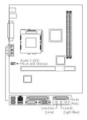
synthesizer, etc. Connect a stereo cable from the line-out jack of your external device to this line-in jack.
