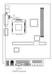
connector J5. Mount the card-edge bracket to the system chassis.
