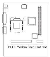
The longer slot (without the shorter one) is a PCI slot. You can install a PCI add-on card into this slot only if the system board is installed in a microATX chassis.
