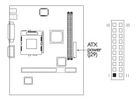
The pin assignment of the ATX power connector is shown below.
