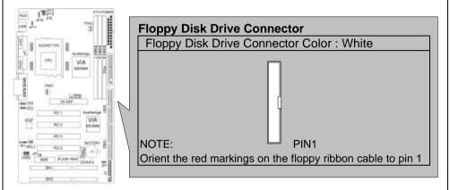
Note: Pin 5 is removed to prevent the users inserting the Floppy Disk Drive in the wrong orientation when using ribbon cables with pin 5 plugged.
