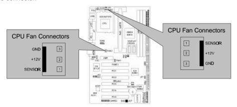
Note: The CPU and motherboard will overheat if there is noairflow across the CPU and onboard heatsink. Damage may occur to the motherboard and the CPU fan if these pins are incorrectly used. These are not jumpers, do not place jumper caps over these pins.
