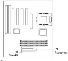
2 Install the other 40-pin header connector(s) into the device with the colored edge of the ribbon cable aligned with pin I of the drive edge connector(s).
