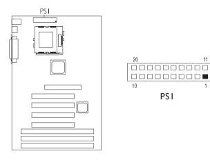
The pin assignment of the ATX power connector is shown below.
