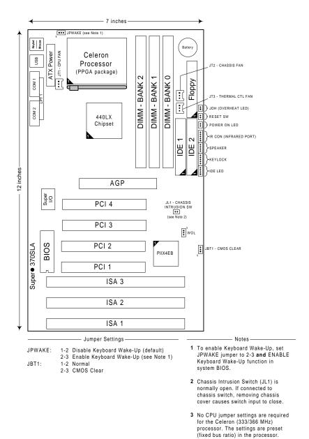
Figure 1-6. SUPER 370SLA Motherboard Layout
