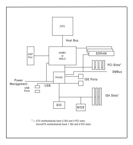
Figure 1-9. 440BX/LX AGP SET: System Block Diagram (Single Processor)
