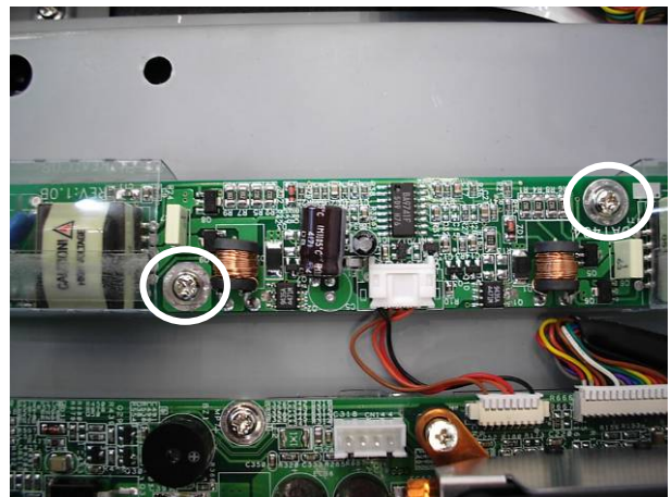
b. Remove the screws (2).
