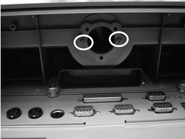
c. Tighten the screws (2) under the pole.
