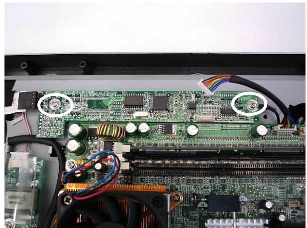
b. Remove the screws (2).
