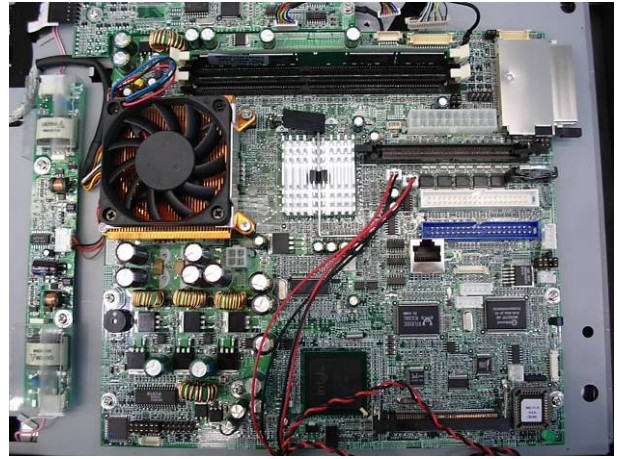
j. Remove the screws (8) of the mainboard.
