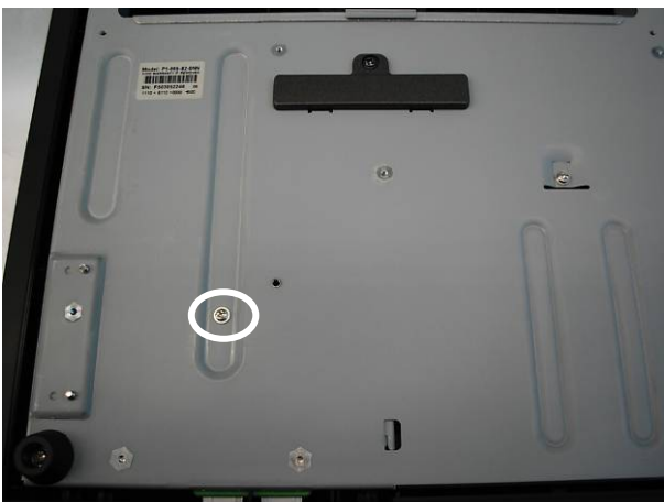
c. Remove the screw (1).
