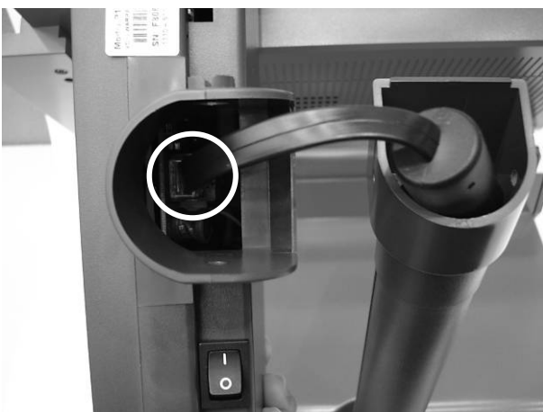
e. Connect the cable into the display.
