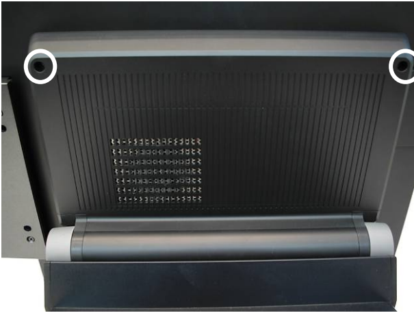
a. Remove the screws (2).
