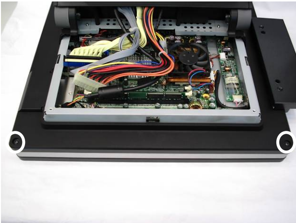
e. Remove the screws (2).
