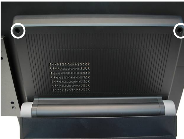
a. Remove the screws (2).
