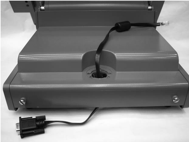
a. Pass the cable through the hole.
