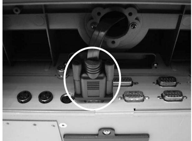
d. Connect the cable. Please setup the COM port power.
