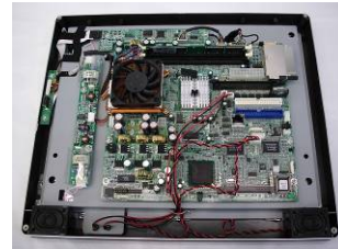
f. Use your hands to carefully press in the two sides to separate the LCD chassis from the base (including LCD cover).
