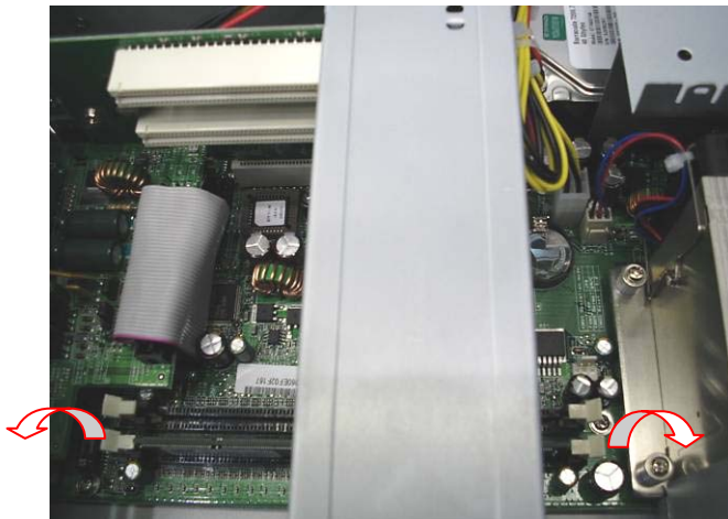
a. Use your finger to push the DIMM slot ejector clips into the down position.
