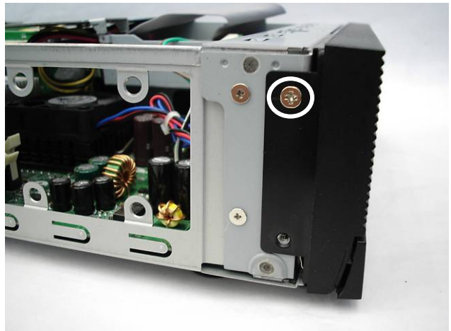
b. Remove the screw (1).
