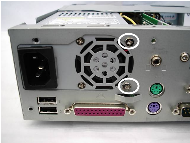
a. Remove the screws (2).
