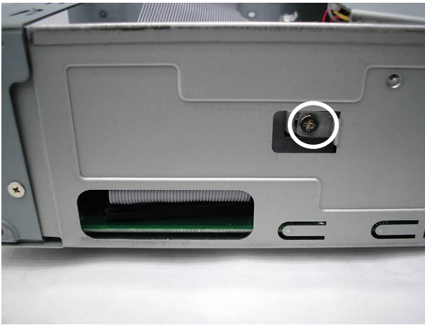
e. Remove the screw (1).
