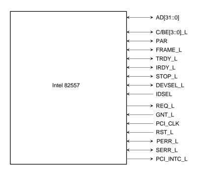
Figure 2-13 Embedded NIC PCI Signals
