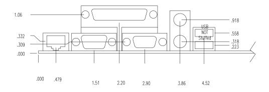
Figure 6-4I/O Connector Mechanical Diagram
