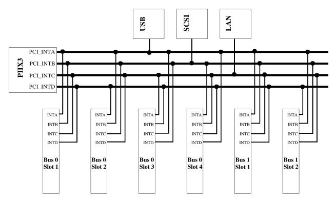
Figure 2-8 PCI Interrupt Routing
