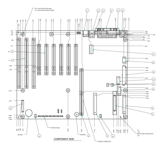
Figure 6-2Baseboard Mechanical Diagram
