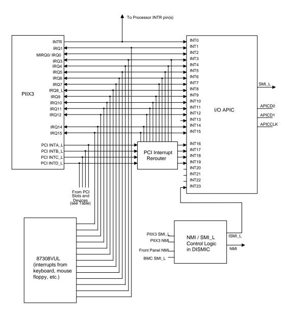
Figure 2-9 Interrupt Connections
