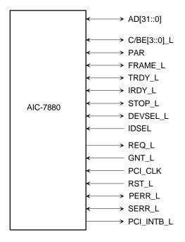
Figure 2-10 Embedded SCSI PCI Signals
