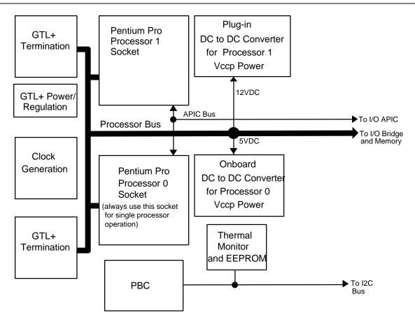
Figure 2-3 Processor Subsystem Block Diagram
