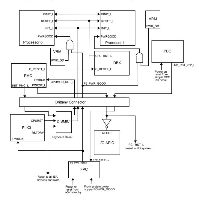
Figure 2-16 System Reset Flow
