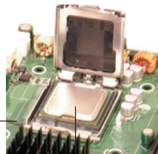
CPU in the CPU socket
