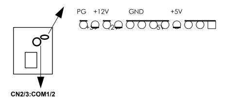
**CN2/CN3**: this two connectors are used to connect serial port cables.
