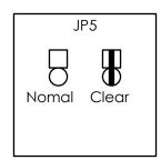
should clear CMOS under powering on, otherwise the 'clear' will not work.
