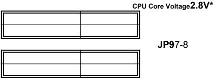
\*Currently, Intel P55C is released 2.8V core voltage only. Please confirm this with your system supplier before you install P55C CPU.
