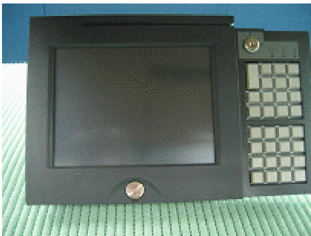
i. Now the keypad is fully installed.
