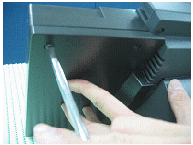
h. Attach the keypad to the side of the system and tighten the four screws around the back cover.
