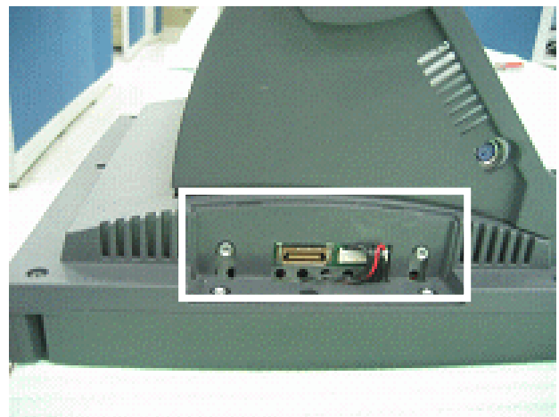
b. Loosen the two screws at the side of the system and remove the keypad cover.
