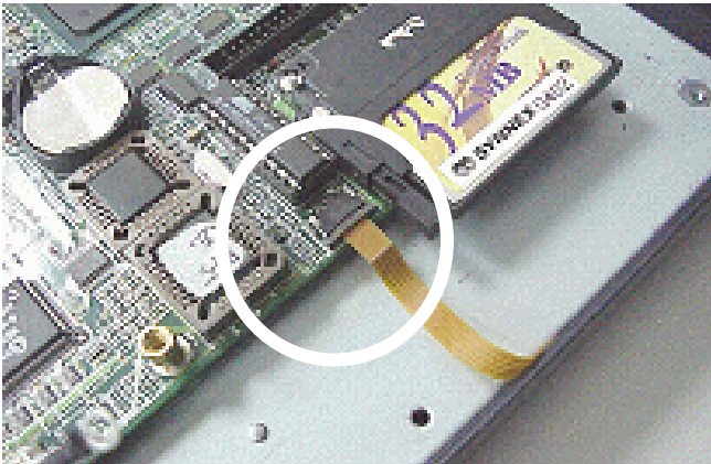
v. Disconnect the touch panel cable.
