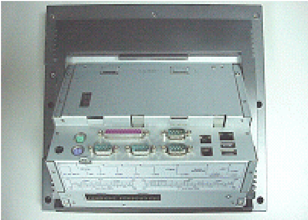
i. Loosen the screws fastening the LCD panel rear cover and the panel to remove it.
