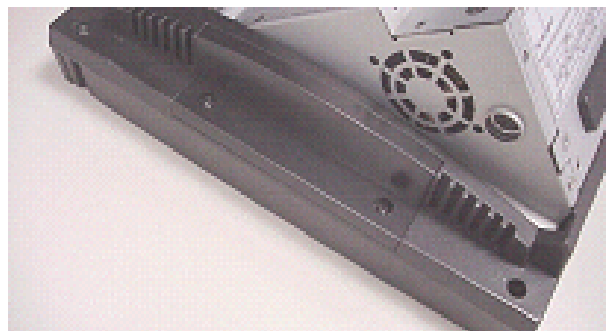
g. Remove the keypad cover and loosen the screw fastening the LCD panel rear cover and LCD panel.
