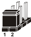
Jumper Block 1-2 pin close(enabled) Looks like this
