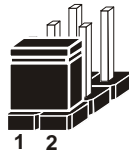
Jumper Block 1-2 pin close(enabled) Looks like this
