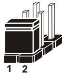
Jumper Block 1-2 pin close(enabled) Looks like this
