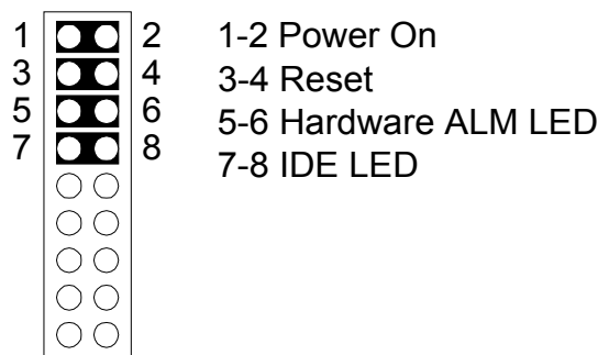
Figure 3-12: Multi-function connector
