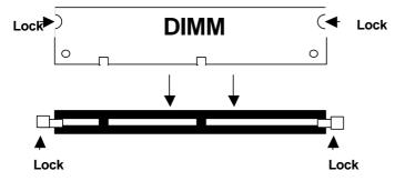
**Top View of DIMM Socket**
