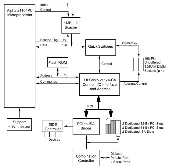
Figure 1–1 AlphaPC 164SX Functional Block Diagram
