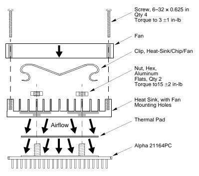
Figure 5–1 Fan/Heat-Sink Assembly
