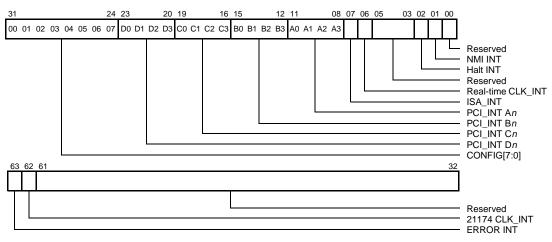
Figure 4–5 Interrupt Request Register
