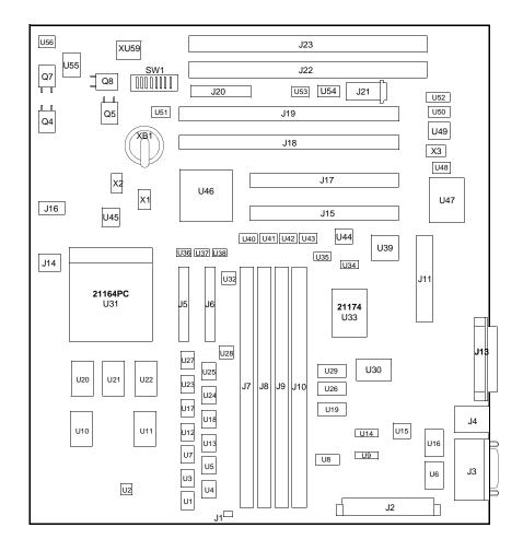
Figure 2–1 AlphaPC 164SX Switch/Connector/Component Location
