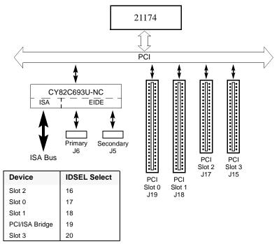
The PCI bus supports multiplexed, burst mode, read and write transfers. It supports synchronous operation of 33 MHz. It also supports either a 32-bit or 64-bit data path with 32-bit device support in the 64-bit configuration. Depending upon the configuration and operating frequencies, the PCI bus supports up to 264-MB/s (33 MHz, 64-bit) peak throughput. The PCI provides parity on address and data cycles. Three physical address spaces are supported:
