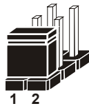
Jumper Block 1-2 pin close(enabled) Looks like this
