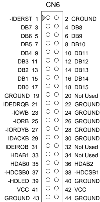
Figure 3-12 CN6: Hard Disk (IDE) Connector
