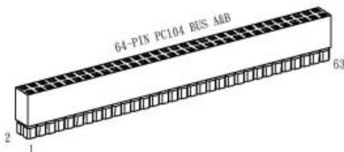
Figure 3-8 CN8: 64 Pin PC/104 Connector Bus A & B
