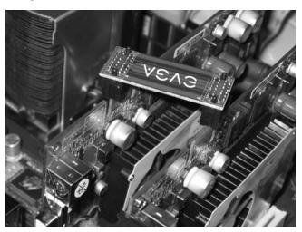
**STEP 4** - Plug the SLI Bridge adapter onto both of the NVIDIA SLI Supported VGA Cards
