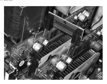
$\mbox{\bf STEP 3}$  - Be careful with the pins as to not damage the adapter or graphics cards during installation.
