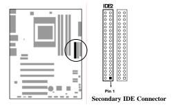
Two hard disks can be connected to each connector. The first HDD is referred to as the "Master" and the second HDD is referred to as the "Slave".
