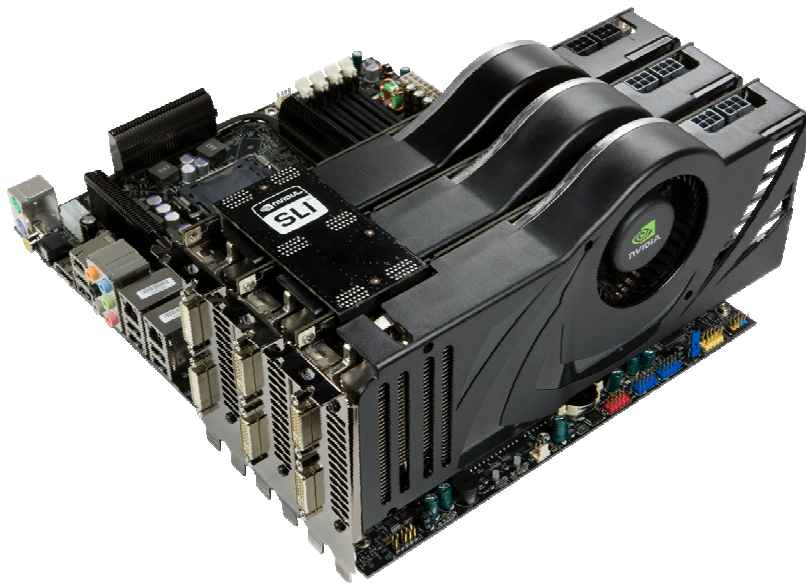
Figure 17. 3-Way SLI Using GeForce 8800 Ultra
