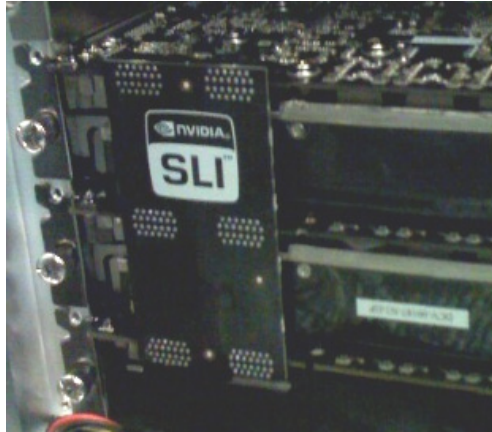
Figure 18. 3-way NVIDIA SLI connector (600-10732-0000-000)
