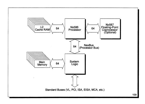
Figure 17 Nx586 based System Diagram
