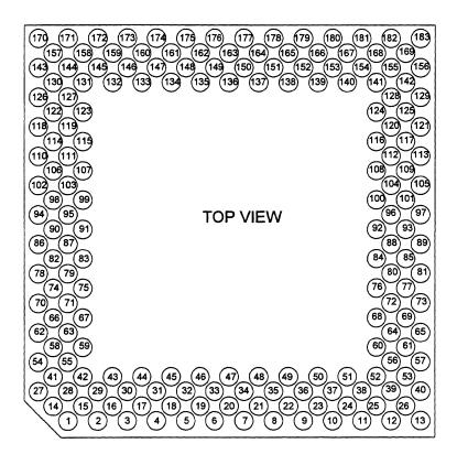
Figure 15 Nx587 Pinout Diagram (Top View)
