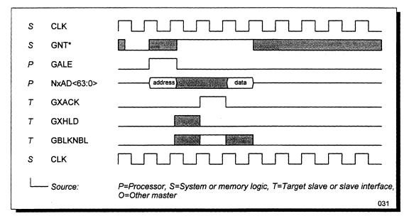
Figure 33 Fastest Single-Qword Write
