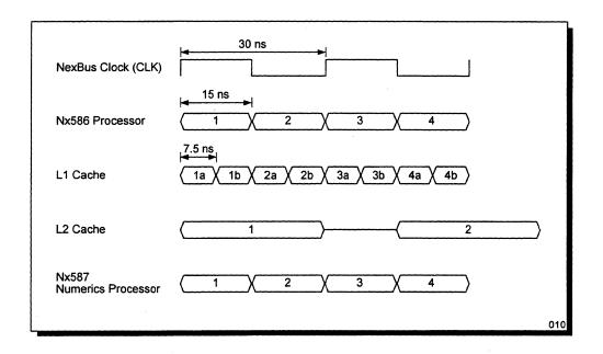
Figure 19 Operating Frequencies (66MHz Processor)
