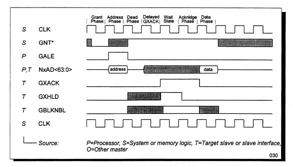
Figure 31 Single-Qword Read with Wait States using a delayed GXACK
