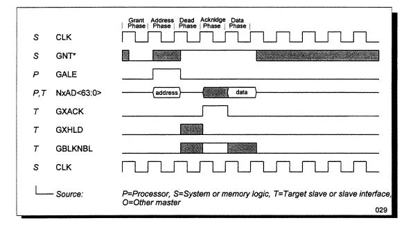
Figure 29 Fastest Single-Qword Read
