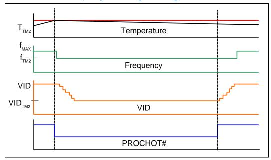
Figure 19. Thermal Monitor 2 Frequency and Voltage Ordering
