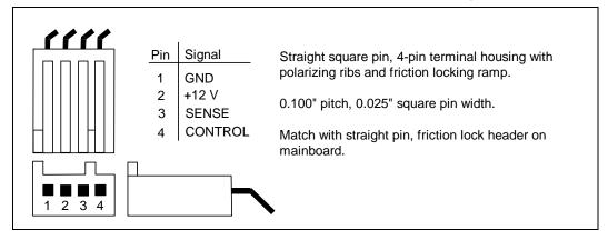
Table 32. **Fan Heatsink Power and Signal Specifications**
