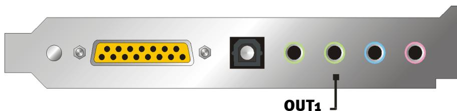
With HiFi amplifiers there are various inputs that are suitable for connecting the card. So you can, for example, keep an eye out for a connector labeled AUX, TAPE (Play), CD, or VIDEO. However, a phono input cannot be used.
