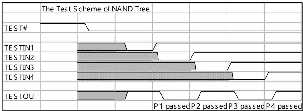
Figure 6.5-4 The Test Scheme of NAND Tree
