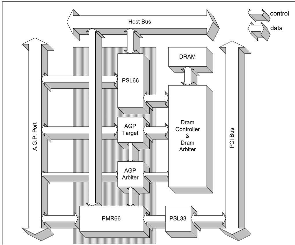
Figure 6.5-1 Block Diagram of AGP Compliant Target/Host-to-PCI66 Bridge
