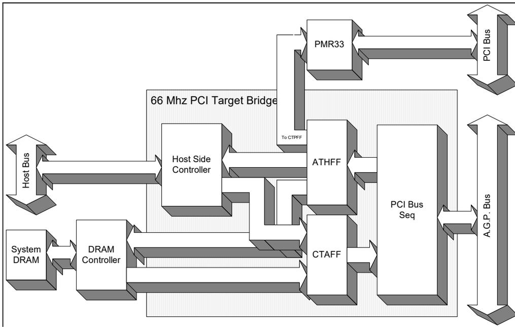
Figure 6.4-9 Block Diagram of 66Mhz PCI Target Bridge
