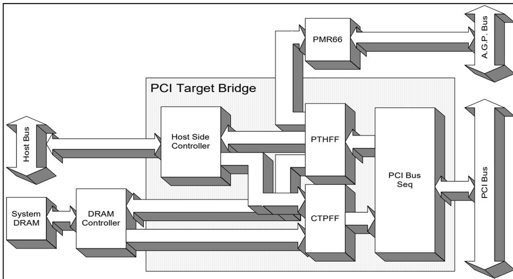
Figure 6.4-4 Block Diagram of PCI Target Bridge
