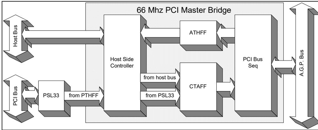
Figure 6.4-3 Block diagram of 66Mhz PCI Master Bridge
