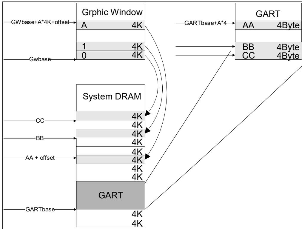
Figure 6.3-5 Graphic Address Re-mapping Function
