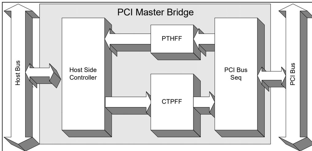
Figure 6.4-2 Block Diagram of PCI Master Bridge
