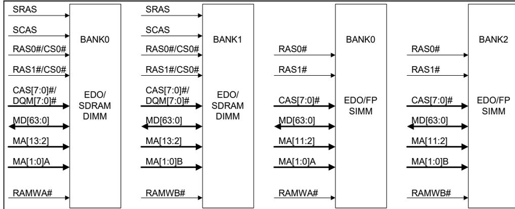
Figure 6.3-3 DRAM Type Mixed Configuration : EDO/FPM + SDRAM
