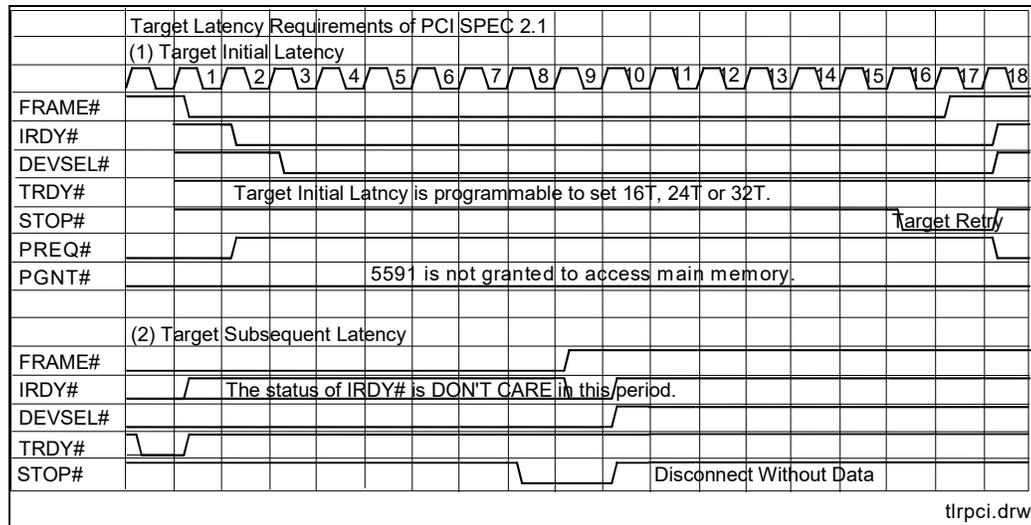
Figure 6.4-5 Disconnect without Data
