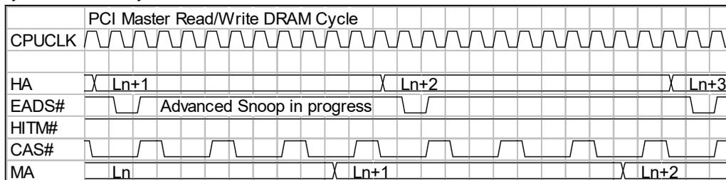
Figure 6.4-6 PCI Master Read/Write DRAM Cycle
