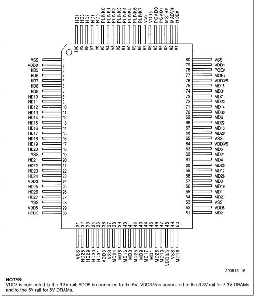
Figure 14. 82438FX Pin Assignment
