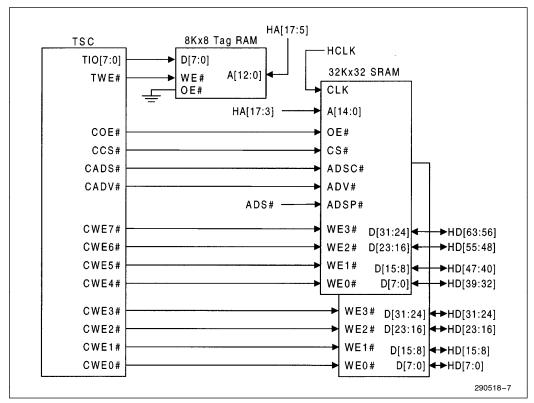
Figure 5. 256-Kbyte Second Level Cache (Burst SRAM)
