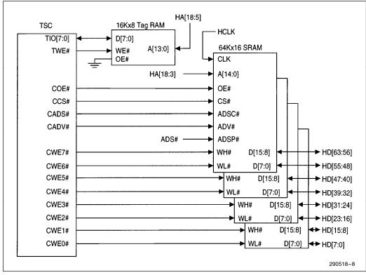
Figure 6. 512-Kbyte Second Level Cache (Burst SRAM)
