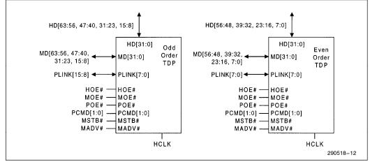
Figure 10. TDP 64-Bit Data Path Partitioning
