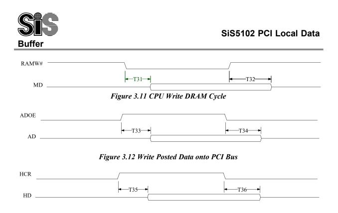
Figure 3.13 CPU Read DRAM or PCI Cycle
