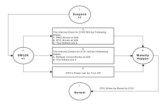
Figure 4.3 Leakage Function Flow Chart
