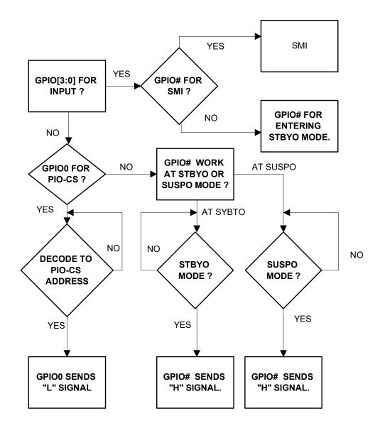
Figure 4.8 SiS5100 GPIO Flow Chart
