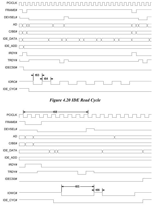
Figure 4.21 IDE Write Cycle
